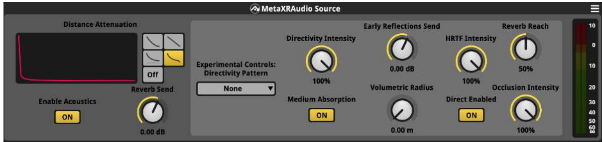
Figure 25: The Meta Spatializer plugin in FMOD controlling HRTF on each spatialized sound giving control over reverb and distance attenuation
