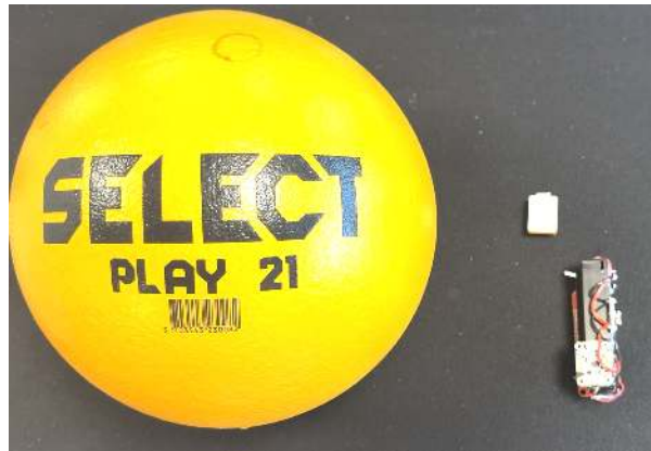
Figure 17: Usecase 2 with the acces point and IMU sensor unit and the ball to place the sensor into
