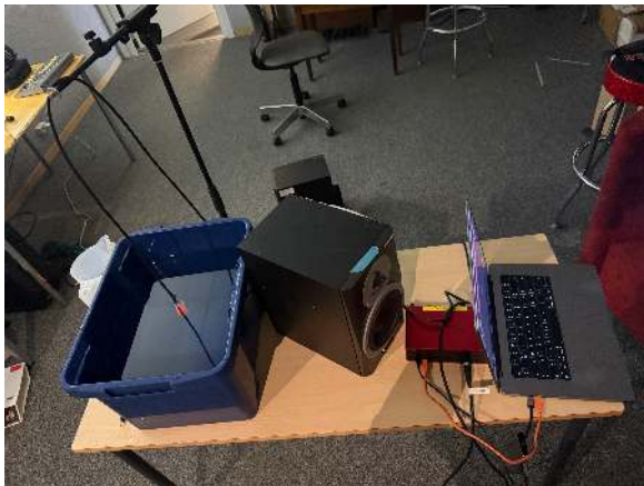
Figure 9: We created a underwater mic from a piezo and recorded the monstersound and the underwater environment
